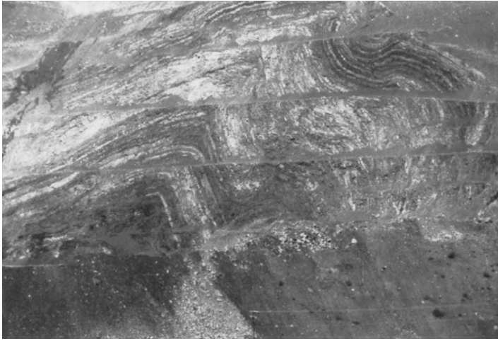
Figure 6.1 Open-pit workings of coal at Lethbridge, British Columbia, note the overturned fold running through the benches.
