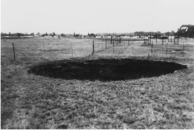
Figure 2.12 A crown hole formed at the surface due to void migration from shallow workings in coal at Springs, South Africa.
