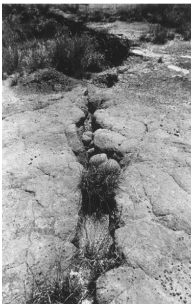
Figure 2.10b A tension crack running from an area that has subsided as a result of pillar failure, Witbank Coalfield, South Africa.
