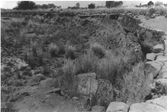
Figure 2.10a Subsidence at the surface caused by pillar failure in shallow abandoned workings, Witbank Coalfield, South Africa.
